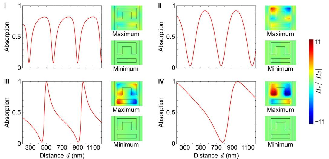
**Figure 3. Metadevice absorption at the metasurface absorption maxima.** Dependence of absorption on the metasurface-to-mirror spacing  $d$  at wavelengths of (I) 615 nm, (II) 785 nm, (III) 930 nm and (IV) 1600 nm. Colour maps show the instantaneous magnetic field  $H_z$  10 nm above the gold surface relative to the incident wave's magnetic field amplitude  $|H_0|$  for absorption maxima and minima.
