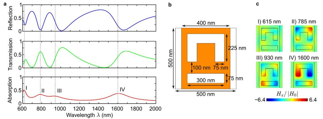
**Figure 2. The metamaterial and its resonances.** (a) Reflection, transmission and absorption of the flat metasurface without mirror. (b) Schematic of the unit cell. (c) Modes of excitation at the absorption maxima in terms of the instantaneous magnetic field  $H_z$  10 nm above the gold surface relative to the incident wave's magnetic field amplitude  $|H_0|$ .
