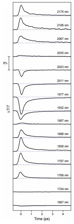
Fig. 2. Spectrally resolved transient changes of transmission of the CNT metamaterial. Pump fluence is 10  $\mu J/cm^2$  (power density – 50 MW/cm²).
