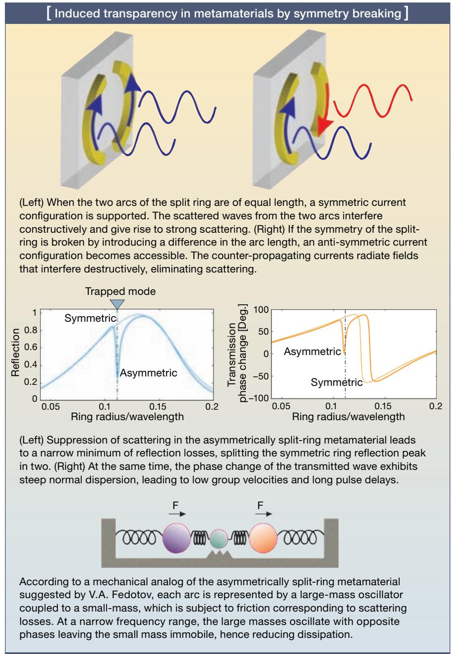
The small mass is also subject to friction, while the two large-mass oscillators are lossless. The system is excited by an external force acting on both large-mass oscillators, representing the incident electromagnetic wave, while friction stands
