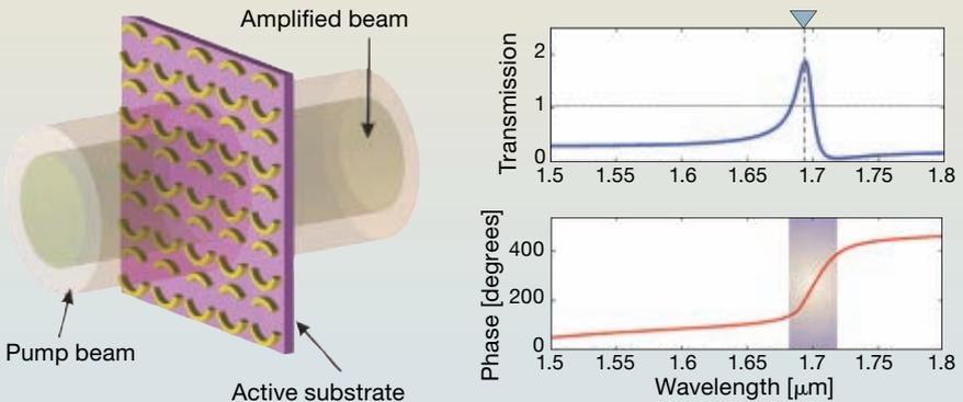
Loss-compensated slow-light device: metamaterial array with EIT-like dispersion placed on a gain substrate ( $\epsilon=9.5+0.35i$ ). At the wavelength of 1.7  $\mu\text{m}$ , it shows single-pass amplification and simultaneously sharp normal dispersion.
