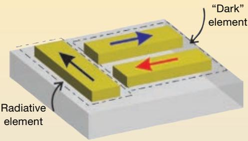
A composite "plasmonic molecule" consisting of a radiative, coupled-to-free-space element and a sub-radiant part. The latter can only be excited through near-field interactions with the radiant element. At a specific wavelength, only the "dark" element is excited, leading to a situation very similar to EIT.
