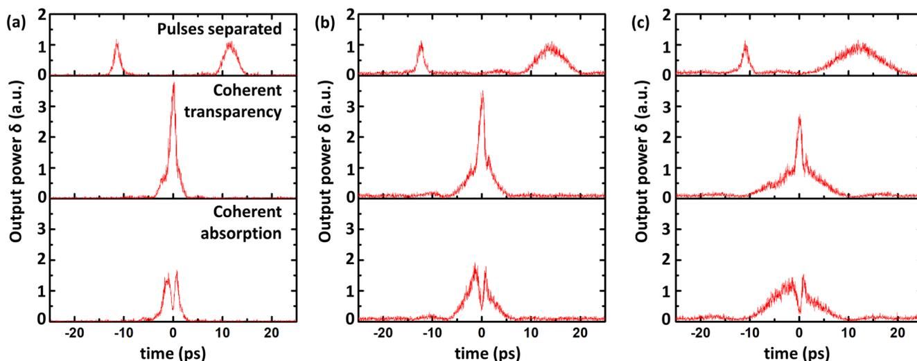
FIG. 5. Generation of 1 ps dark pulses. Output power in channel  $\delta$  in the cases when the input pulses in channels  $\alpha$  and  $\beta$  are separated in time (top); the pulses overlap in the coherent transparency regime (middle); the pulses overlap in the coherent absorption regime (bottom). The columns correspond to different durations of the input pulses in channel  $\beta$  of (a) 3 ps, (b) 6 ps, and (c) 9 ps. In all cases, the duration of the pulses in channel  $\alpha$  was 1 ps.
