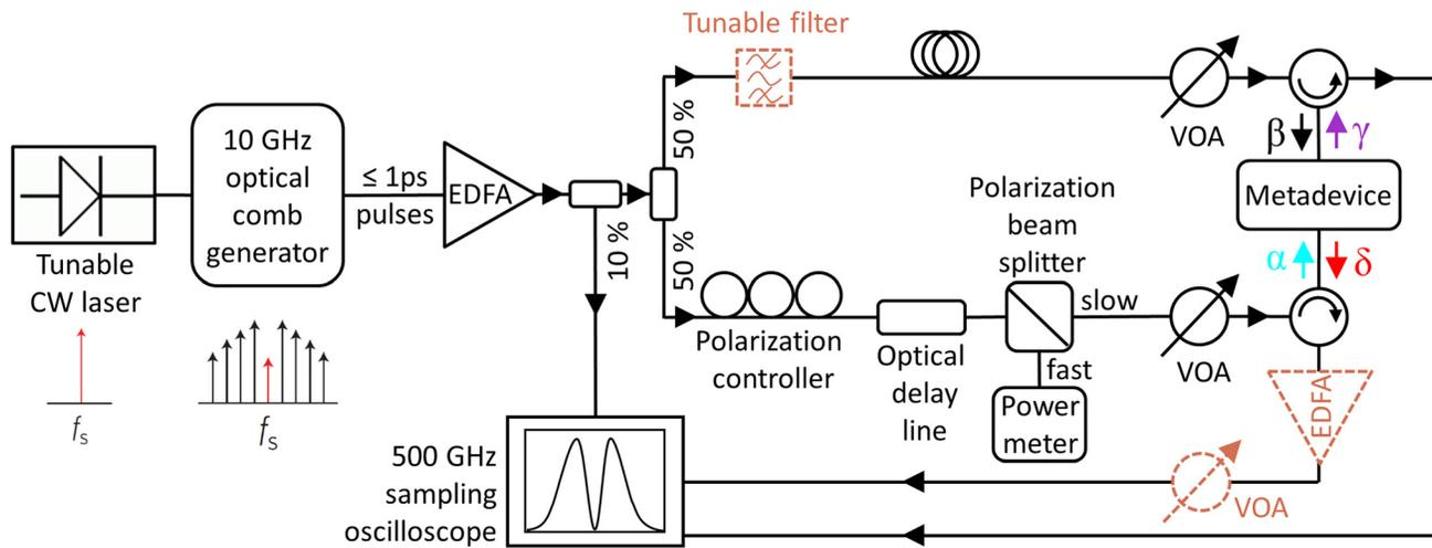
FIG. 2. Coherent signal processing and dark pulse generation. Experimental setup for controlled absorption and transmission of 1 ps pulses (black lines) with additional components required for dark pulse generation and detection (brown dashed lines). VOA—Variable Optical Attenuator; EDFA—Erbium Doped Fibre Amplifier.
