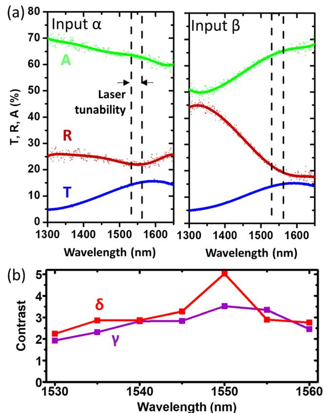
FIG. 4. Broadband signal processing. (a) Metadvice transmission (T), reflection (R), and absorption (A) as measured with light entering the metadvice from either input  $\alpha$  (left) or  $\beta$  (right). The data points are shown with polynomial fits (lines). (b) Modulation contrast observed for output channels  $\gamma$  and  $\delta$  as functions of laser wavelength.
