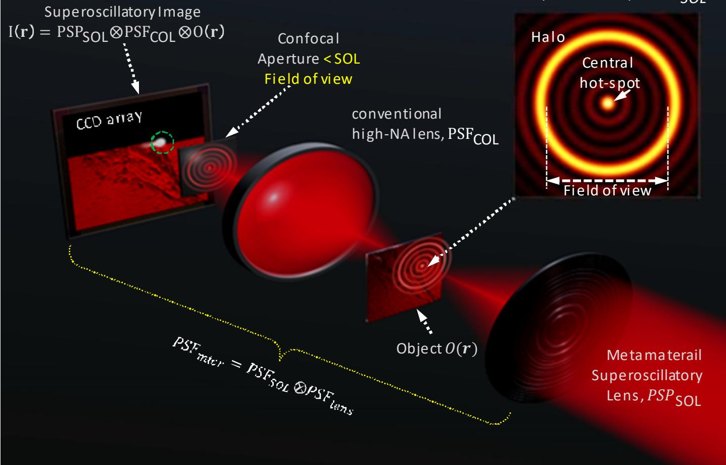
**A super-oscillatory lens optical microscope for subwavelength imaging**
