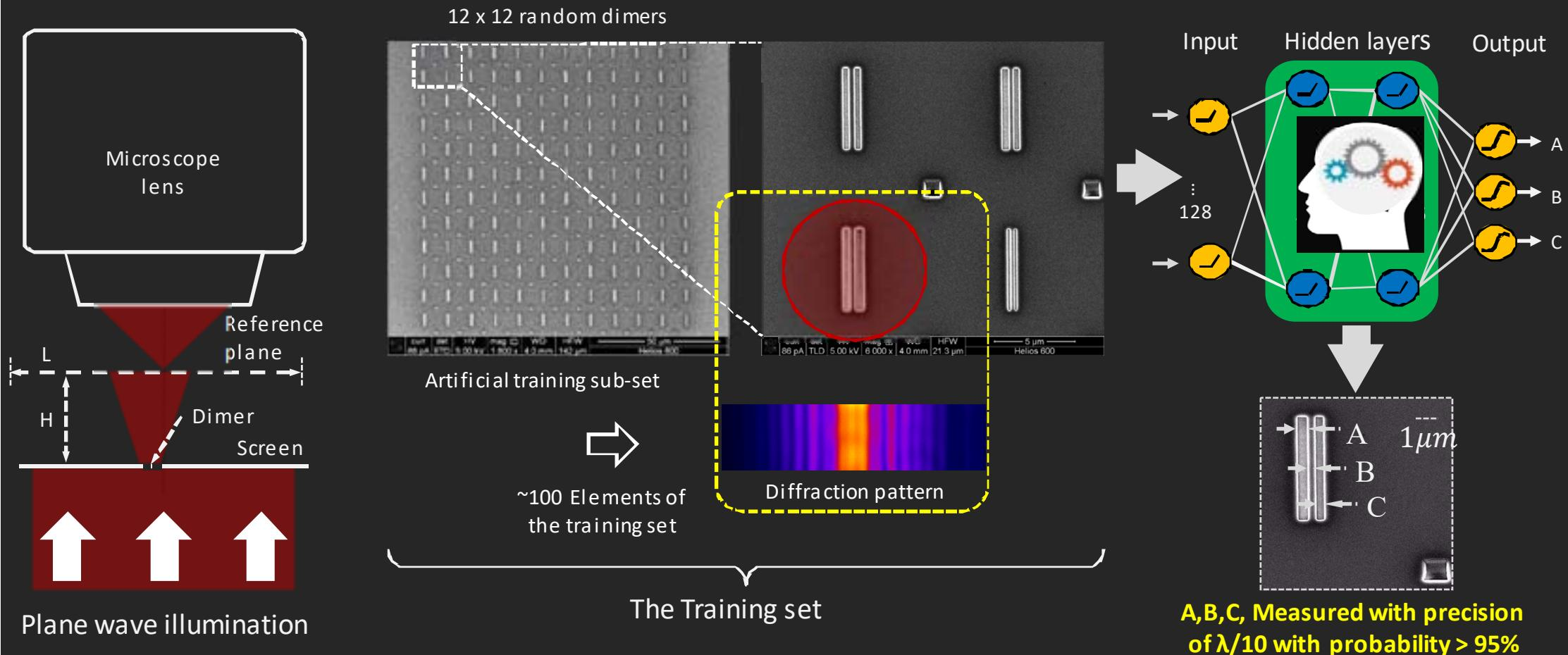
Label-free deeply subwavelength optical microscopy
