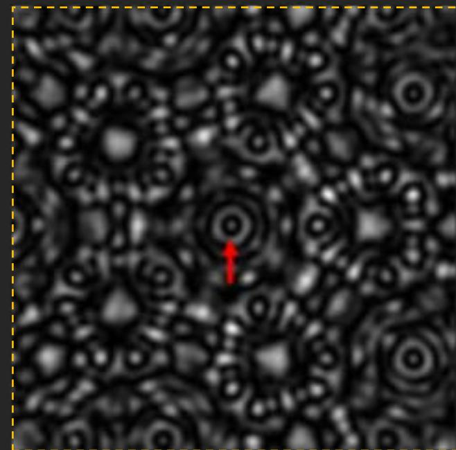
Focusing of light by a nanohole array
