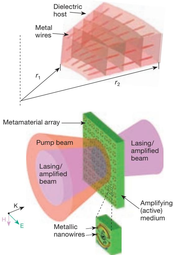
Top: A cylindrical cloak consists of wires that are all perpendicular to the cylinder's inner and outer interfaces. The spatial positions do not have to be periodic. Bottom: The "lasing spaser" structure consists of a gain medium slab (green) supporting a regular array of metallic asymmetric split-ring resonators.
