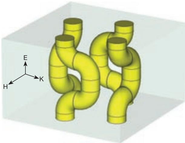
Top: Electron micrographs of photonic metamaterial structures using direct laser writing. Bottom: A photonic metamaterial that can be grown by laser beam deposition. The structure exhibits a negative index along two directions.
