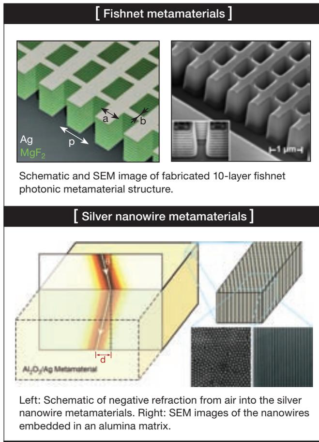
Schematic and SEM image of fabricated 10-layer fishnet photonic metamaterial structure.
