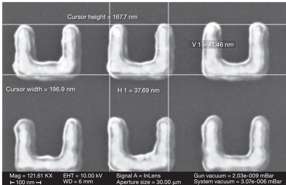
SRR structures: Photo of nanoscale split ring resonator structures fabricated in Bilkent University.
