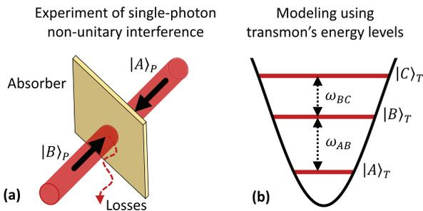
**FIG. 1.** Building a model of the photon interference experiment on a transmon. A correspondence is established between the optical interference experiment with a thin absorber (a) and a transmon of a quantum computer (b): The presence of a photon in the input ports  $|A\rangle_P$  and  $|B\rangle_P$  corresponds to states  $|A\rangle_T$  and  $|B\rangle_T$  of the transmon. Losses are represented by the transition to the excited state  $|C\rangle_T$ .
