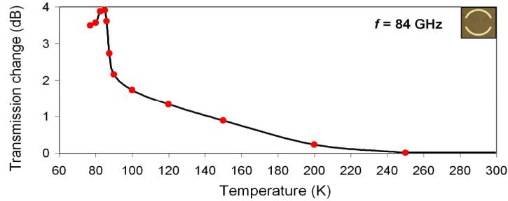
Fig. 3. Change of transmission measured at 84 GHz as a function of temperature for negative superconducting YBCO metamaterial (relative to its room temperature state). Experimental data is presented by red dots, while black curve provides guide for eye.
