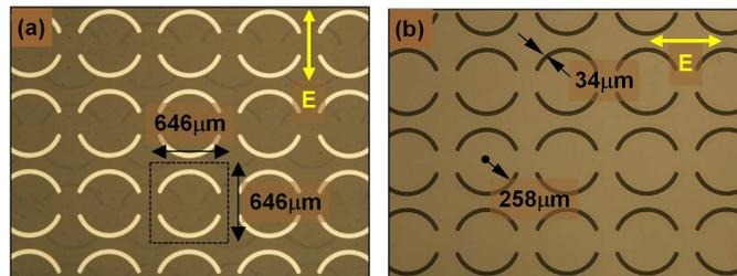
Fig. 1. Superconducting metamaterials. Panels (a) and (b) show photographs of correspondingly negative and positive forms of asymmetrically-split ring metamaterial. Dashed box indicates the metamaterial's unit cell.
