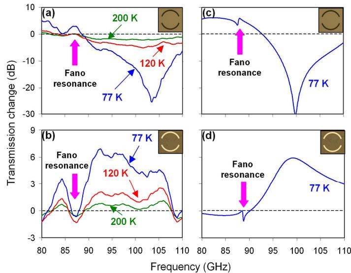
Fig. 2. Changes in transmission spectra of superconducting YBCO metamaterials relative to their room temperature state. Panels (a) and (b) present experimentally measured data for positive and negative metamaterial designs respectively, while panels (c) and (d) show corresponding results of numerical simulations.
