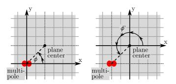
FIG. 5. (Color online) The difference between  $\phi$  and  $\phi'$ . Angle  $\phi$  is defined in the coordinate frame of a multipole under consideration, while the angle  $\phi'$  is defined in the coordinate frame of the multipole array (also see Fig. 2). The observer (see Fig. 2) is located directly above the origin of the array.
