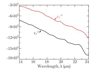
FIG. 9. (Color online) The experimentally measured dielectric constant of the gold used for simulating the case-study metamaterial. The complex-valued dielectric constant is given by  $\tilde{\epsilon}_r = \epsilon'_r + i\epsilon''_r$ .
