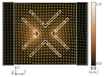
FIG. 10. (Color online) Distribution of magnetic field around the test-case metamolecule at the resonance ( $\lambda = 17.4 \ \mu$ m). The arrow plot shows the direction of magnetic field while the color map on the background shows the magnitude of the field. The regions outside the metamolecule have been partially screened to highlight the unit-cell boundaries.
