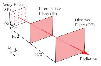
FIG. 7. (Color online) The (emitter) array plane, intermediate plane, and the observer plane used in the proof of validity of Eq. (5). The distances between the neighboring planes are R/2 and the lengths of the rectangular unit cells of the array are  $\Delta x$  and  $\Delta y$ .
