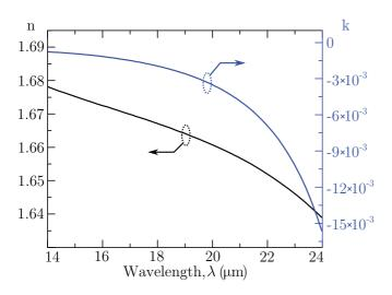
FIG. 8. (Color online) The experimentally measured refractive index of the polymer SU-8 used for simulating the case-study metamaterial. For simulations of the response of metamaterial on Fig. 3, the gold split-ring resonators were embedded into SU-8 polymer. The complex-valued refractive index of SU-8 is given by  $\tilde{n} = n + ik$ .
