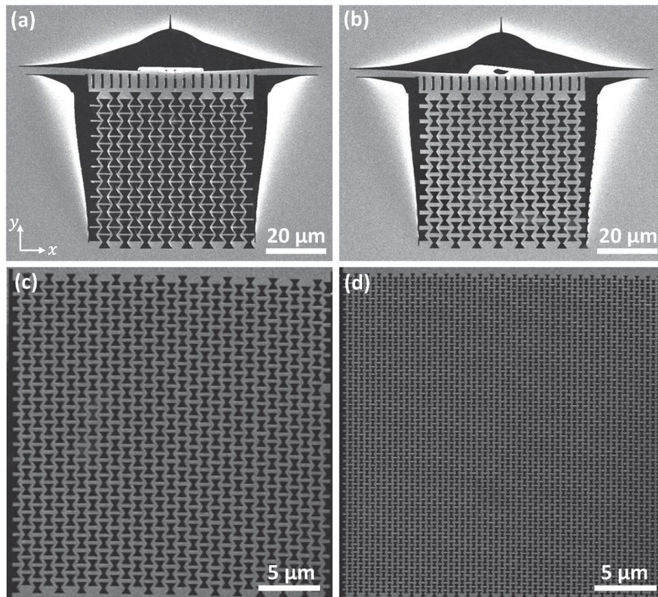
**Figure 2.** a–d) Scalable design of auxetic metamaterial with different dimensions of the rectangular cell:  $7\ \mu\text{m} \times 5\ \mu\text{m}$  (a,b),  $1.8\ \mu\text{m} \times 1.2\ \mu\text{m}$  (c), and  $900\ \text{nm} \times 600\ \text{nm}$  (d). All structures are fabricated from a  $110\ \text{nm}$ -thick gold-coated silicon nitride membrane.
