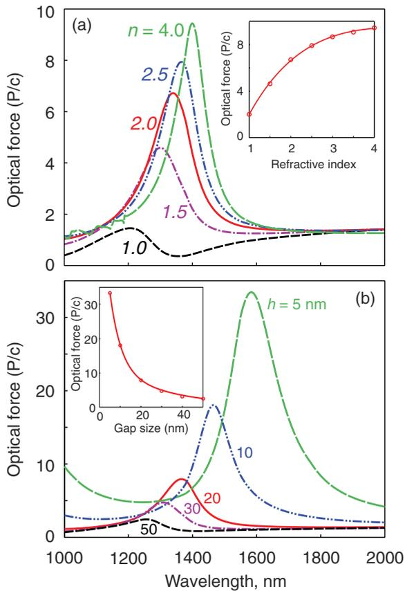
FIG. 3. (Color online) Optical forces between a plasmonic metamaterial and a dielectric surface. Spectral dispersion of the total optical force [under illumination from free space as illustrated inset to Fig. 2(b)] for different values, as labeled, of (a) dielectric refractive index  $n$  (at  $h = 20$  nm) and (b) gap size  $h$  ( $n = 2.5$ ). Insets show peak optical force as a function of  $n$  and  $h$ , respectively.
