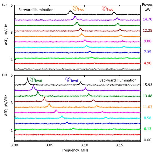
**Figure 2.** Optical control of nanowire Eigenfrequencies. Transmission amplitude spectral density, showing peaks ① and ② as assigned in Figure 1c, for opposing directions of light propagation through the sample (a) forward and (b) backward [light incident respectively on the silicon and the silicon nitride side], and for a range of laser power levels [as labeled].
