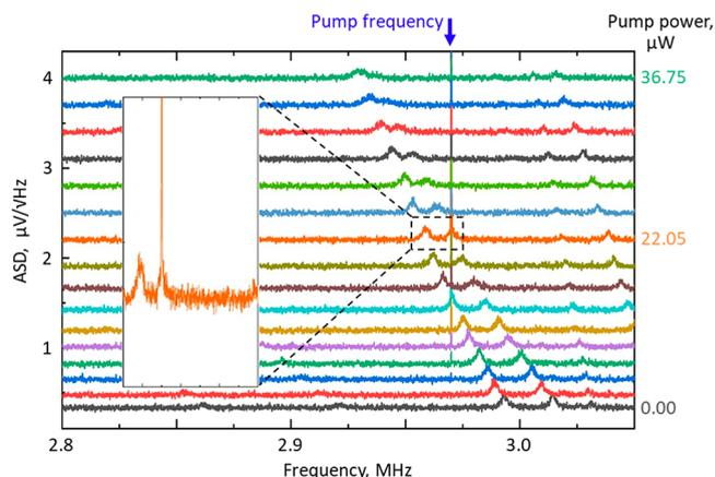
**Figure 4.** Optical control of nanomechanical motion: thermal and nonthermal mechanisms. Amplitude spectral density of probe transmission (in the forward direction) for a range of pump peak power levels with a fixed pump modulation frequency.
