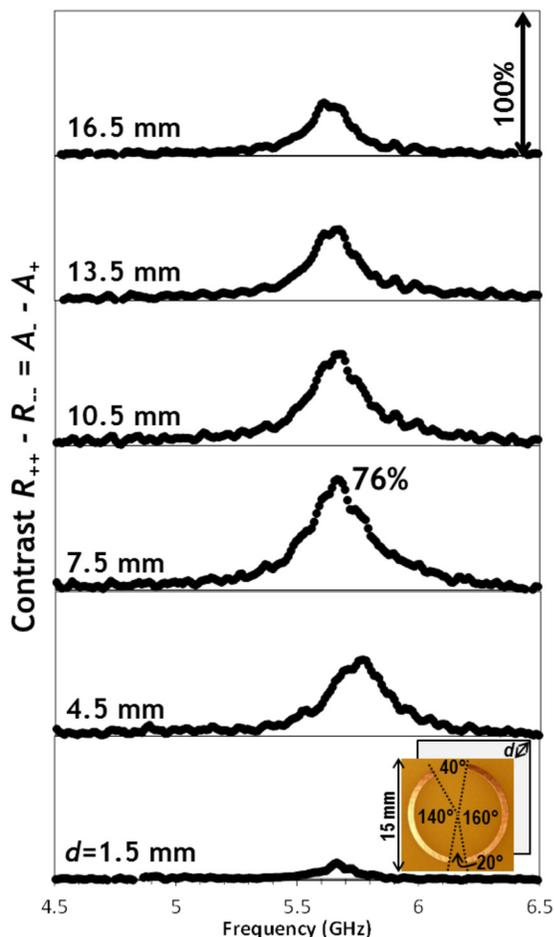
FIG. 3. Polarization contrast of an RCP mirror as a function of the spacing  $d$  between split rings and aluminum plate.
