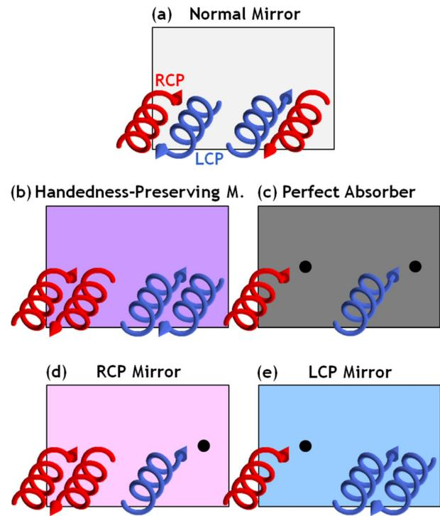
FIG. 1. Mirrors. (a) A conventional mirror reverses the handedness of circularly polarized waves. (b) Structures designed to reflect  $x$  and  $y$  polarizations with a phase difference of  $\pi$  act as handedness-preserving mirrors.<sup>8</sup> (c) Perfect absorbers do not reflect. Here, we demonstrate (d) RCP and (e) LCP mirrors, which reflect circularly polarized waves of one handedness without handedness reversal, while absorbing the other.
