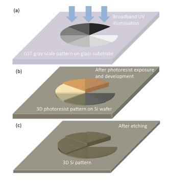
FIG. 1. Sketch of the 3D spiral phase plate fabrication process. (a) Grayscale photomask is prepared by direct optical writing in a GST thin film. (b) The photoresist is exposed and developed leaving a 3D photoresist structure on the substrate. (c) 3D silicon structure is obtained by uniform etching of the substrate and remaining photoresist.
