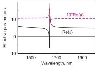
Fig. 6. Silicon metamaterial near-IR magnetic response. (a) Spectral dispersion of effective permittivity  $\epsilon$  and permeability  $\mu$  derived from simulated scattering data for the zero-loss asymmetric metamaterial model structure of Fig. 2(a) under normally incident x-polarized illumination [N.B. the amplitude of permeability is multiplied here by a factor of ten for visibility on the same scale as permittivity].
